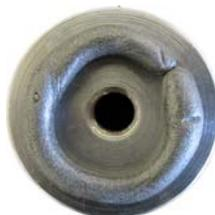
Push the pad with glue to the prepared place and, while constantly pushing and turning the pad there and back with circular movements, observe that the cement is being evenly pushed out along the circumference of the pad. The purpose is to make the layer between the pad and the surface as thin as possible.
