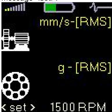
Push arrows, it changes the value of speed with the step 250 RPM. When the correct speed ( or the value near the correct speed) is defined, push Enter button for confirmation.
