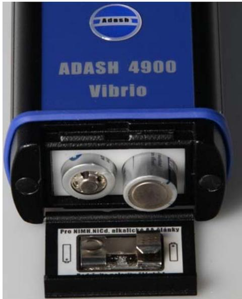
Fig. Placement of power batteries
