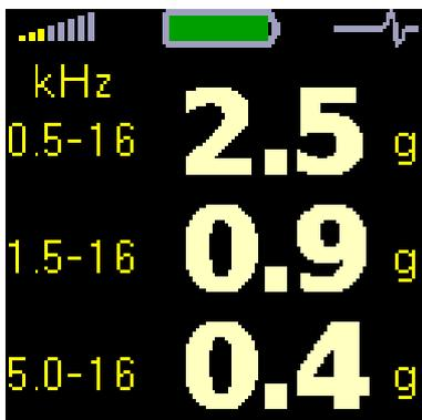
The last screen shows a case, when the vibration may not be excited by a bearing or a gear. Very often these are vibrations of the equipment tied to the mentioned machine. In case of multiple-geared transmissions, however, these can be also the tooth frequencies of the second or third transmission gear. Here we would not be able to do without a detailed analysis, using an instrument with possibility of the spectrum analysis measurement.
