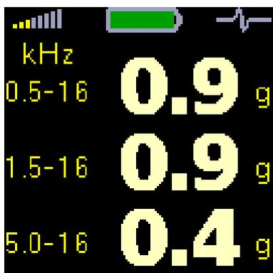
**Vibrations in frequency ranges – gearbox/bearing**
